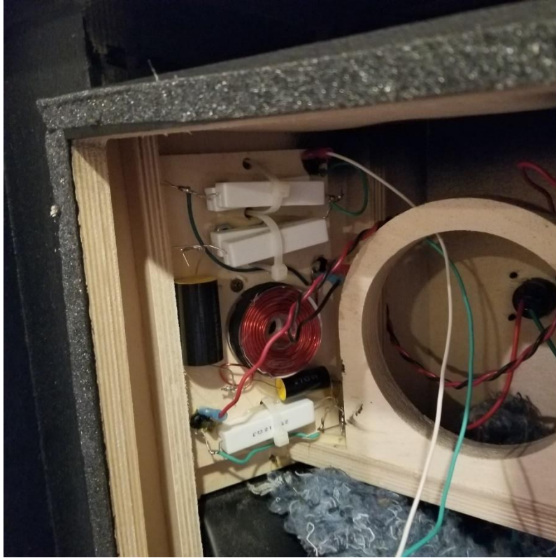
Figure 14 Tweeter Crossover Location (note, I keep them away from stuffing material)
