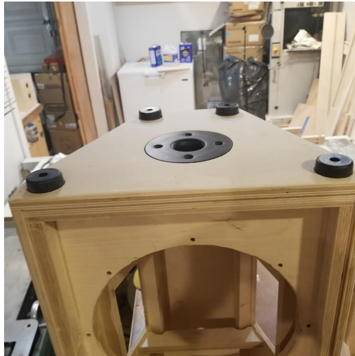
Figure 9 Pole Mount and Foot Detail
